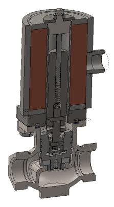
When the normally closed value is energized, flow occurs from the inlet to outlet. When deenergized, flow stops. The value will only stop a fluid in the direction of inlet to outlet. It does not stop fluid from moving in the reverse direction, i.e.  $P_{inlet}$  must be greater than or equal to  $P_{oulet}$  at all times to prevent back flow.
