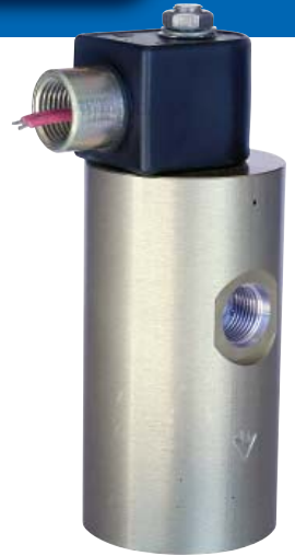
EH50 Series, 1/2" - Full Port 10,000 PSIG Operating Pressure
