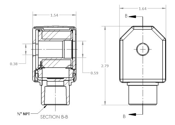
Figure 1 – 10 Series Coil Dimensions
